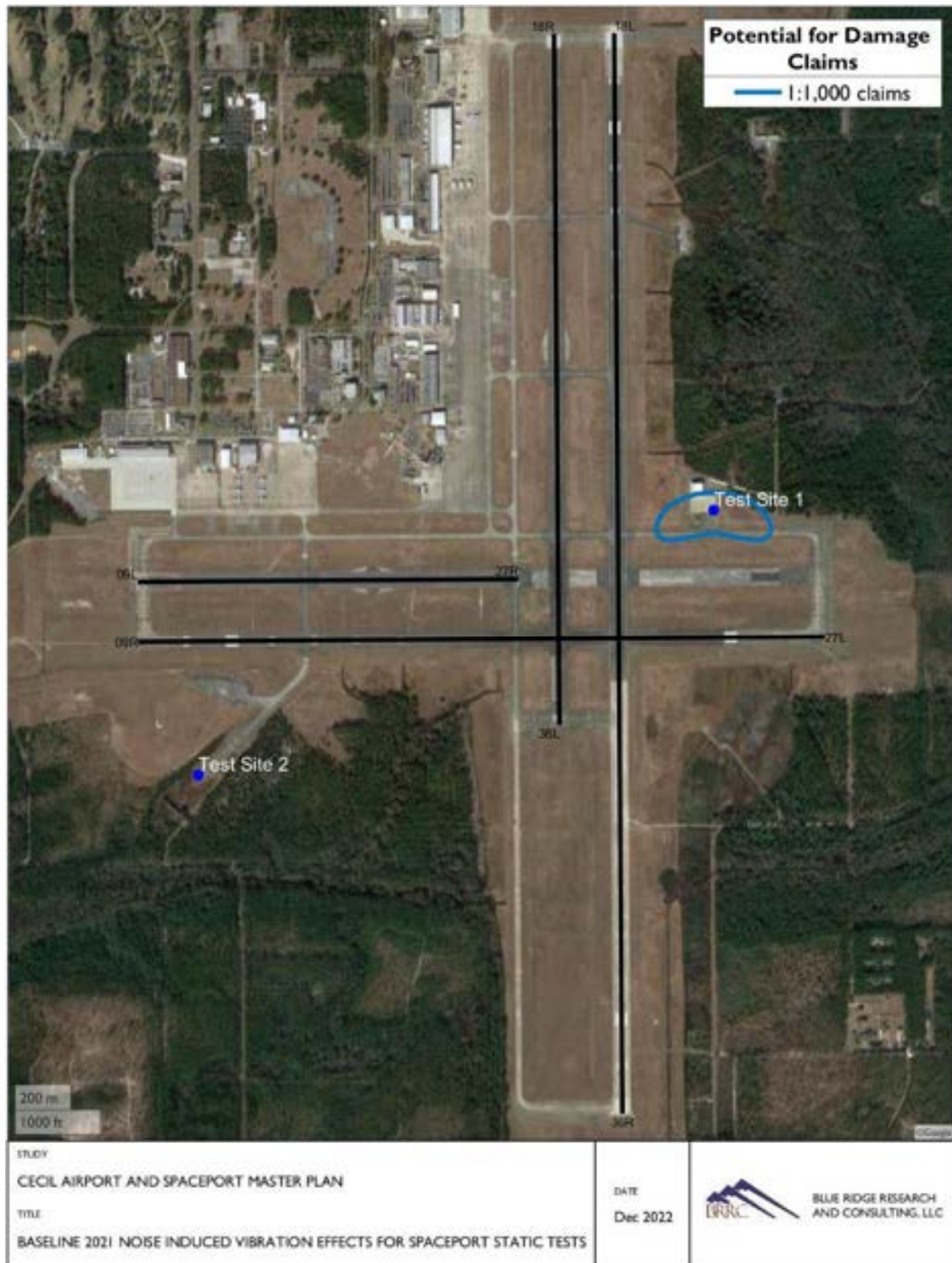
Figure 13. Baseline 2021 Potential for Damage Claims Contours at Cecil Spaceport
